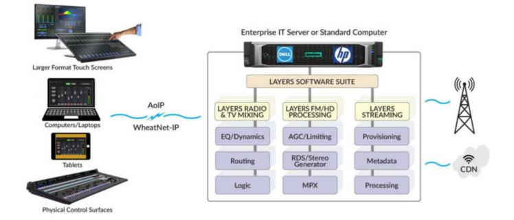
The user can also consolidate several stations and studios into one or two servers; add instances as needed for backend mixing, FM processing, stream provisioning, and metadata management; and backup WheatNet-IP studios in a redundant server on or offsite without additional physical studios required.
